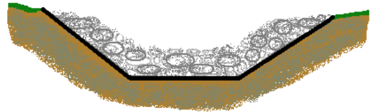
Cross section of an open limestone channel
